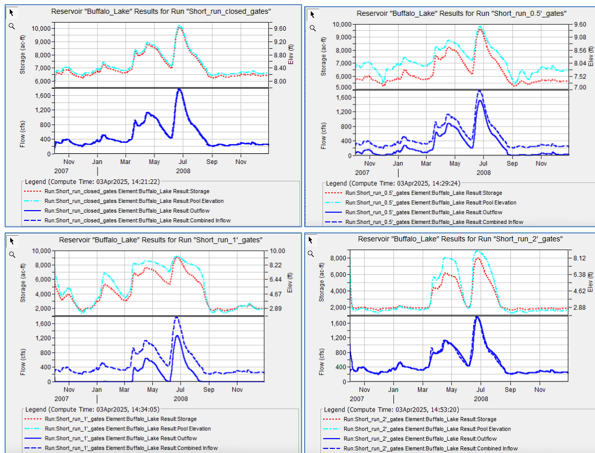
Figure 5. HEC-HMS simulation of 2007-2008 flows for gates closed (upper left), gates open 0.5 ft (upper right), gates open 1.0 ft (lower left) and gates open 2.0 ft (lower right). Lake stage shown in light blue.
